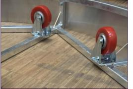
The roller system is designed with a fully closed lifetime lubricated center bearing supported by 10 wheels with a diameter of 125mm. The outer wheels ensures a smooth rotation under heavy load.
